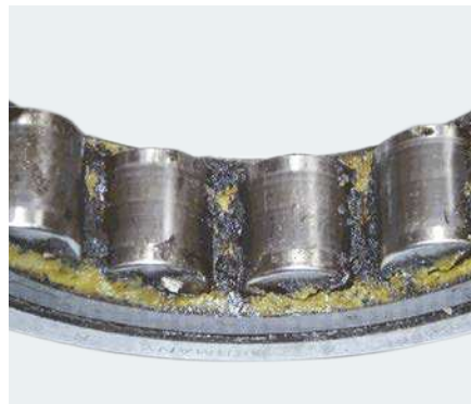
Cylindrical roller bearing outer ring with cage, rollers and grease: current leakage resulted in burnt grease (black) on the cage bars
